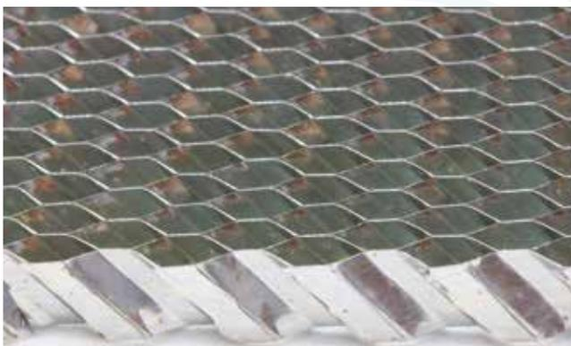
Kemtron's standard honeycomb vent uses 2 layers of 1/8" cell X 1/4" thick laid at 90°, this is known as cross cell. Cross cell honeycomb improves shielding performance by eliminating any polarising effects.
